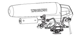
2. When assembling it with camera or DSLR, insert the cold shoe into the slot of the camera. Turn the knob clockwise to fix the microphone. When assembling it with photography stand, connect the 1/4 socket on the microphone with photography stand. Turn it clockwise to fix the microphone.
