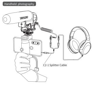
5. When connecting with camera or DSLR for recording, it is recommended to set the mic volume fader to 0dB. When connecting with cell phone for recording, it is recommended to set the mic volume fader to +10dB.
